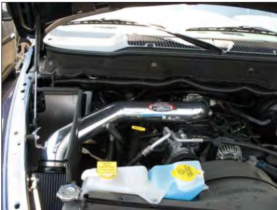
AEM® intake system installed
