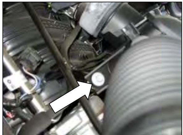
d. Loosen and remove the mounting bolt to the intake plenum.
