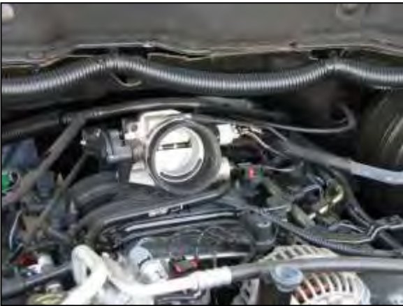
h. Attach the coupler to the throttle body and secure with the #56 hose clamp.
