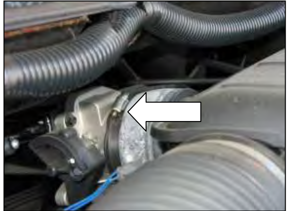
b. Loosen the hose clamp at the throttle body.
