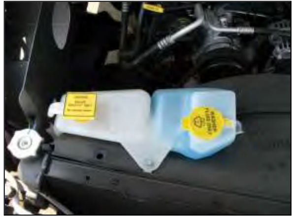
g. Reinstall the washer/coolant overflow reservoir.
