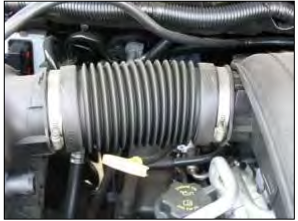
f. Loosen the hose clamp at the intake plenum.
