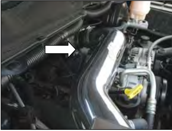
o. Reattach the IAT sensor harness connector.
