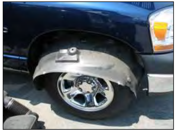
h. Remove the fender liner on the passenger side to access the air box mount.
