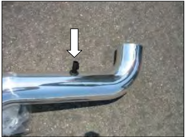
k. Insert the IAT sensor into the inlet pipe
