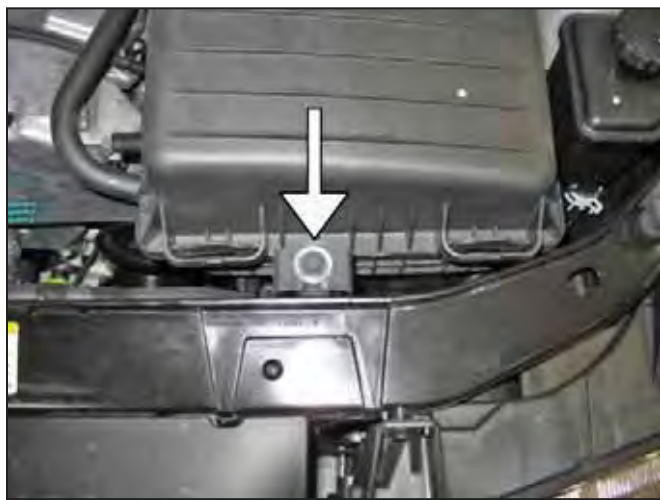
d. Loosen and remove the air box mounting screw. This screw will be reused.
