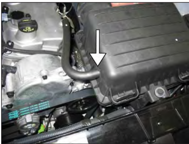
c. Remove the PCV breather tube from the air box.
