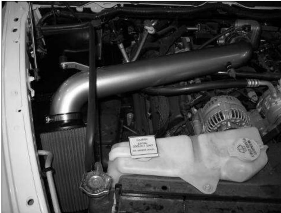
AEM® intake system installed
