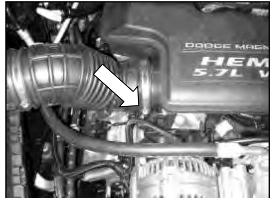
b. Loosen the hose clamp at the intake air resonator. Remove the rubber air hose and the air box lid.
