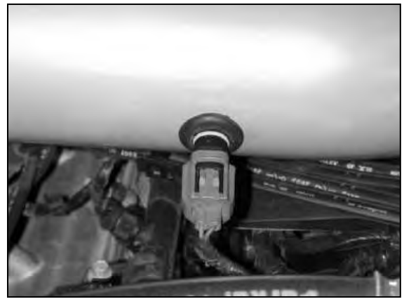
p. Reconnect the wire harness to the IAT sensor. Do not push the grommet through the pipe.
