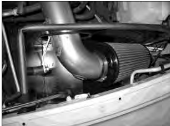
s. Install the air filter from inside the fender well. Slide the air filter on to the pipe until it stops. Secure with the supplied hose clamp. Make sure the windshield washer wires and hose do not come into contact with the air filter.
