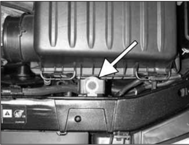
g. Loosen and remove the mounting bolt. This bolt will be reused in a later step. Remove the airbox.
