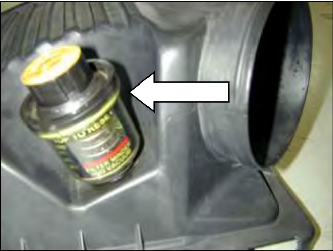
f. Remove filter status meter from upper air box.
