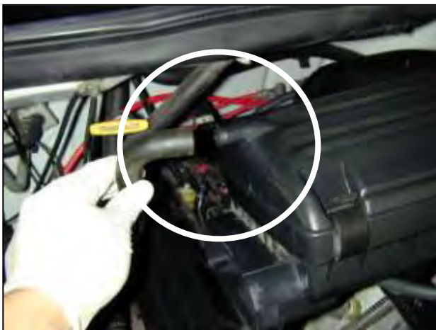
c. Remove the crankcase breather hose from the air filter housing. If the hose is on the passenger side of the air box, the hose may be left connected to the valve cover and will be reused with the AEM® intake system. If the hose is on the driver's side of the air box, remove the entire hose from the engine bay.
