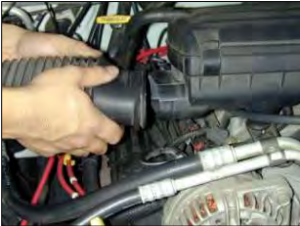
a. Release the air intake tube from the air filter housing by pulling straight back.
