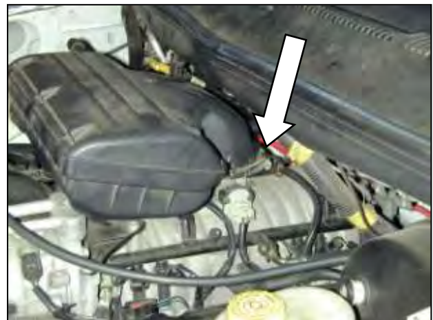
d. Loosen the hose clamp holding the air filter housing to the throttle body. Remove the air filter housing.
