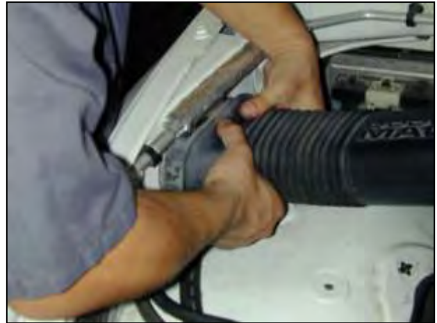
b. Remove the other end of the air intake tube from the inner fender by pulling away while squeezing from the top and bottom.
