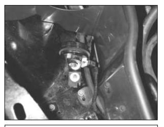
f. Reassemble the upper horn to the new bracket with the factory washer and nut. Secure to the mounting stud with provided nylok nut and washer. The horn should point toward the heat shield. Reattach harness.
