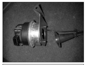
h. Insert the mounting studs of the cruise control unit into the AEM<sup>®</sup> bracket as shown.
