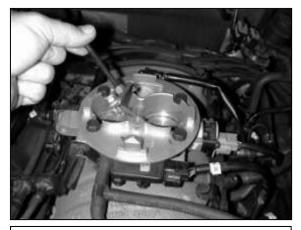
b. Remove the stud assembly from the throttle body.
