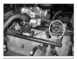
a. Unsnap the cruise control cable from the throttle linkage. Push the cable stop out of the bracket and remove the cable assembly from the throttle body.
