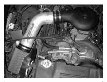
o. Install the air filter on to the end of the intake pipe. Orient the intake so that no parts of the filter or pipe touch the vehicle, wiring, or heat shield. When proper placement is achieved, tighten all three hose clamps and the nut on the rubber mount.
