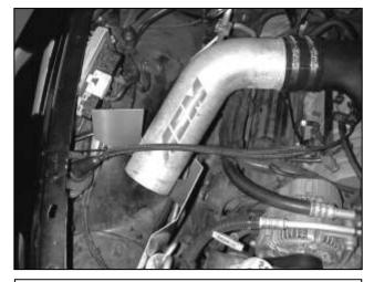
m. Insert the intake pipe as shown in the picture. Do not tighten the hose clamps.
