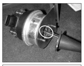
i. Attach the cable to the cruise control unit and re-install the cotter pin.
