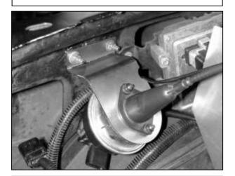
k. Install the cruise control in the vehicle in location of the factory bracket. Secure it in place be re-using 2 of the factory nuts, the third nut will be used to install the heat shield. Plug the cruise control electrical connector in to the unit.
