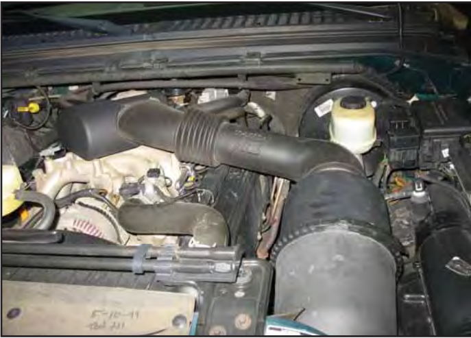
Factory air box system installed
