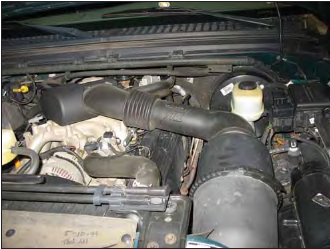
a. Factory air box system installed.
