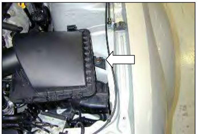
d. Remove the bolt securing the stock air box to the vehicle. Lift up on the stock air box until it is free from the vehicle.
