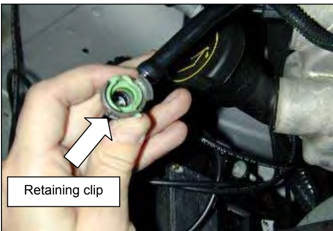
c. Loosen the hose clamp on the throttle body attached to the stock intake hose. Unplug the plastic breather hose connected to the intake hose. This is done by sliding the green retaining clip until the hose is free from the nipple.
