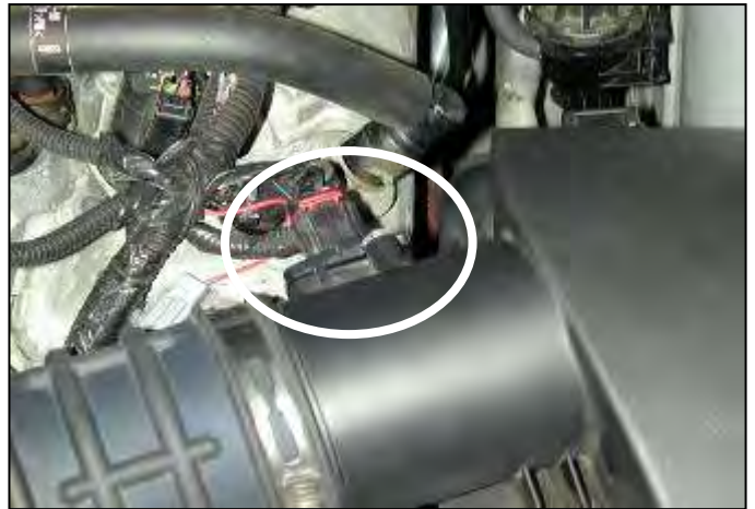
b. Unplug the wire harness from the Mass Air Flow (MAF) sensor.
