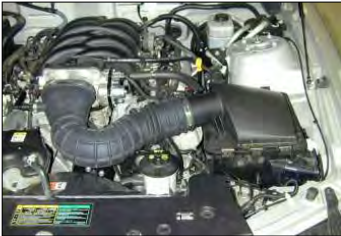
a. Factory air box system installed.
