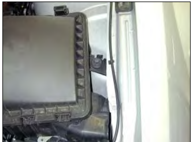
d. Remove the bolt securing the stock airbox to the vehicle. Lift up on the stock airbox until it is free from the vehicle.
