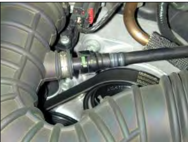
c. Loosen the hose clamp on the throttle body attached to the stock intake hose. Unplug the plastic breather hose connected to the intake hose. This is done by sliding the green retaining clip until the hose is free from the nipple.
