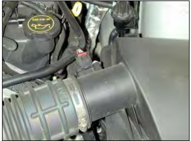
b. Unplug the wire harness from the Mass Air Flow (MAF) sensor.
