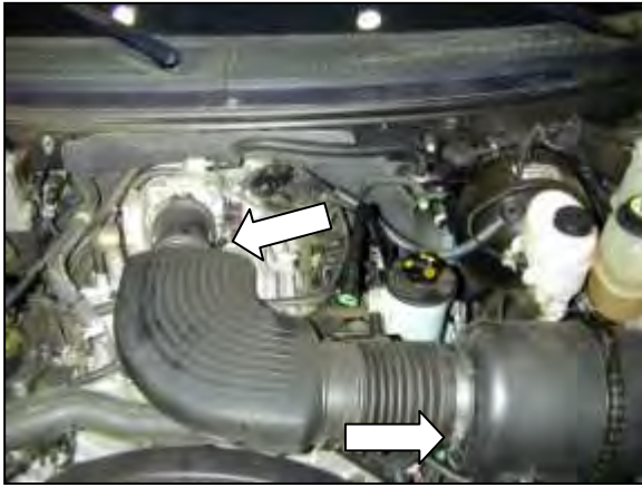
c. Loosen hose clamps at the throttle body and the air filter housing.
