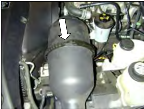
e. Unclasp the clip holding the air filter element casing together.
