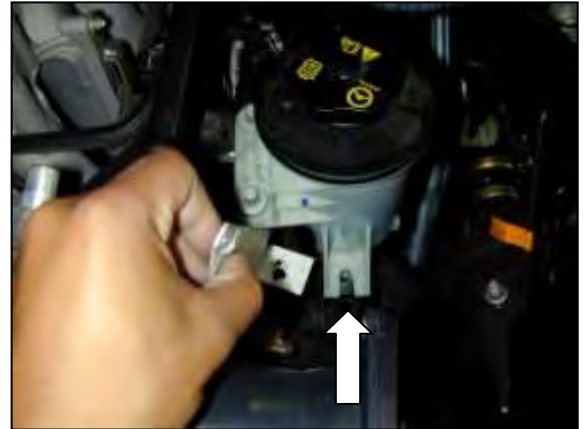
n. Remove the front bolt that secures the power steering fluid reservoir. Loosen the other two bolts. Place the MAF sensor bracket tab under the front tab of the power steering fluid reservoir. Secure mounting position, but do not fully tighten.
