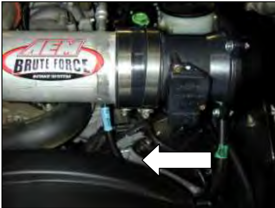
m. Insert the MAF sensor assembly into the coupler. NOTE: Make note of the air flow direction.
