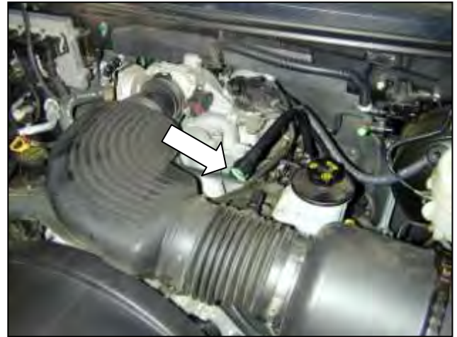
b. Unclip the plastic crankcase breather tube from the stock air inlet tube.
