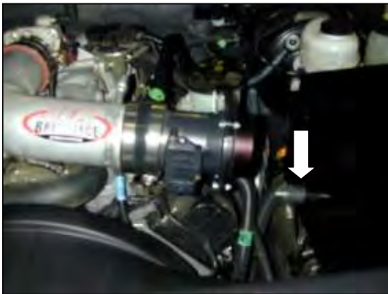
o. Insert rubber mount into the heat shield and secure with provided washer and nylok nut.
