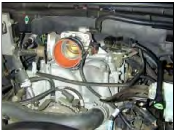
i. Attach the reducer coupler to the throttle body and secure with hose clamp #48. The other end should not be tightened.
