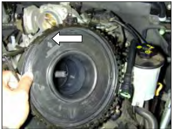
f. Gently pry open the housing at the any one of the tabs. Careful not to damage the MAF sensor.
