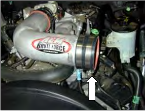
k. Attach and secure the connecting coupler to the upper inlet pipe.
