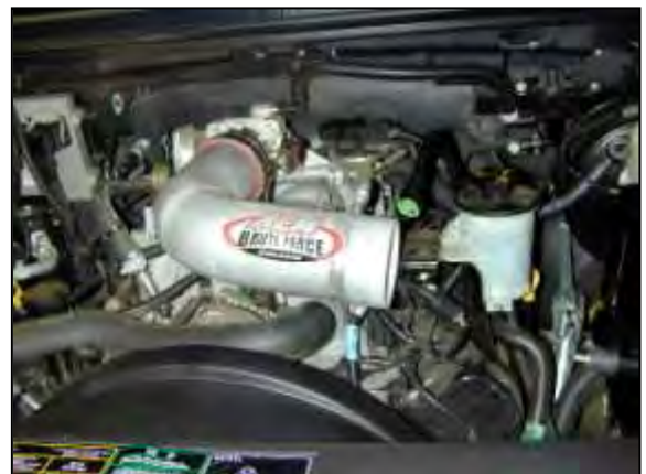
j. Insert the upper inlet pipe into the coupler and secure.
