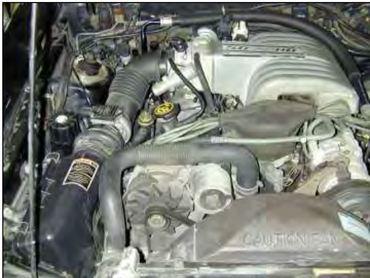
Factory air box system installed
