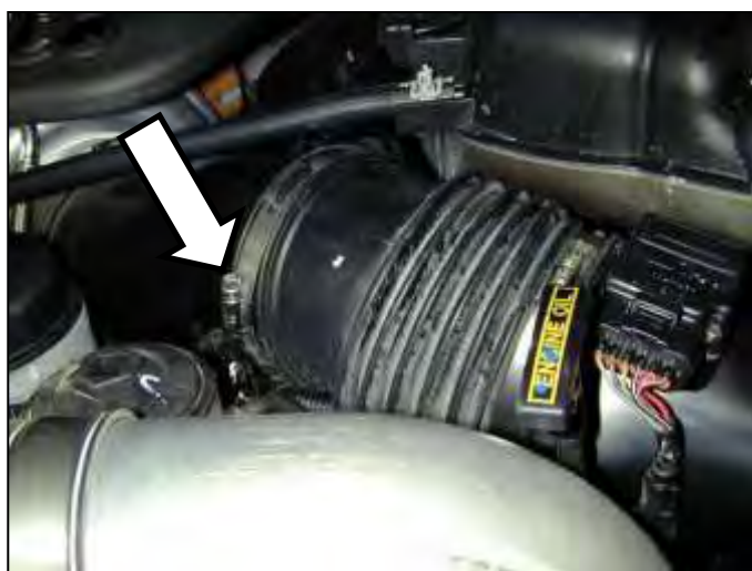
c. Loosen the hose clamp on the turbo inlet pipe.
