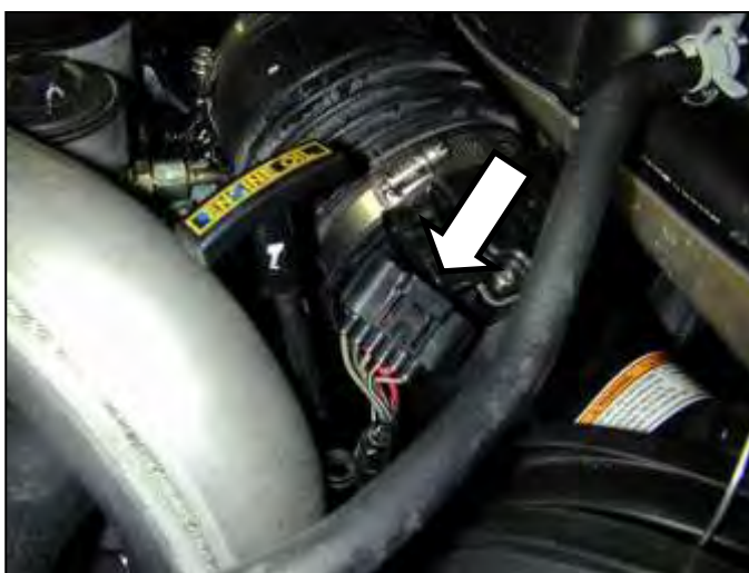
d. Vehicle equipped with MAF sensor. Unplug the mass air flow (MAF) sensor.
