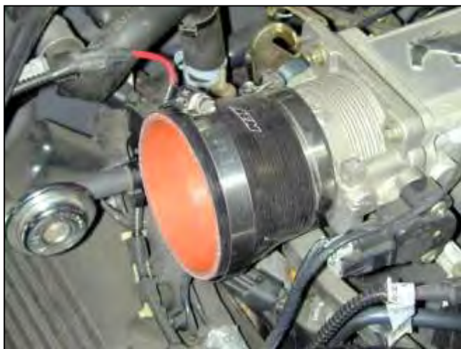
b. Attach reducer coupler and hose clamps. Do not completely tighten.
