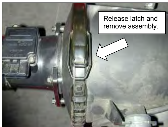
e. Release latch and remove the air filter element and housing.
