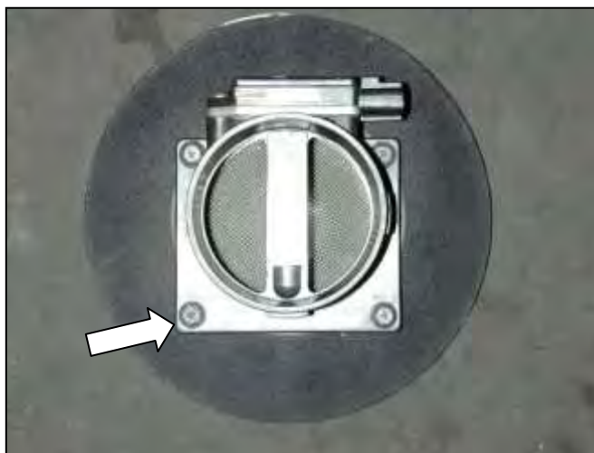
f. Loosen and remove the 4 bolts retaining the MAF sensor. Remove the MAF sensor. The screen will not be reused.
