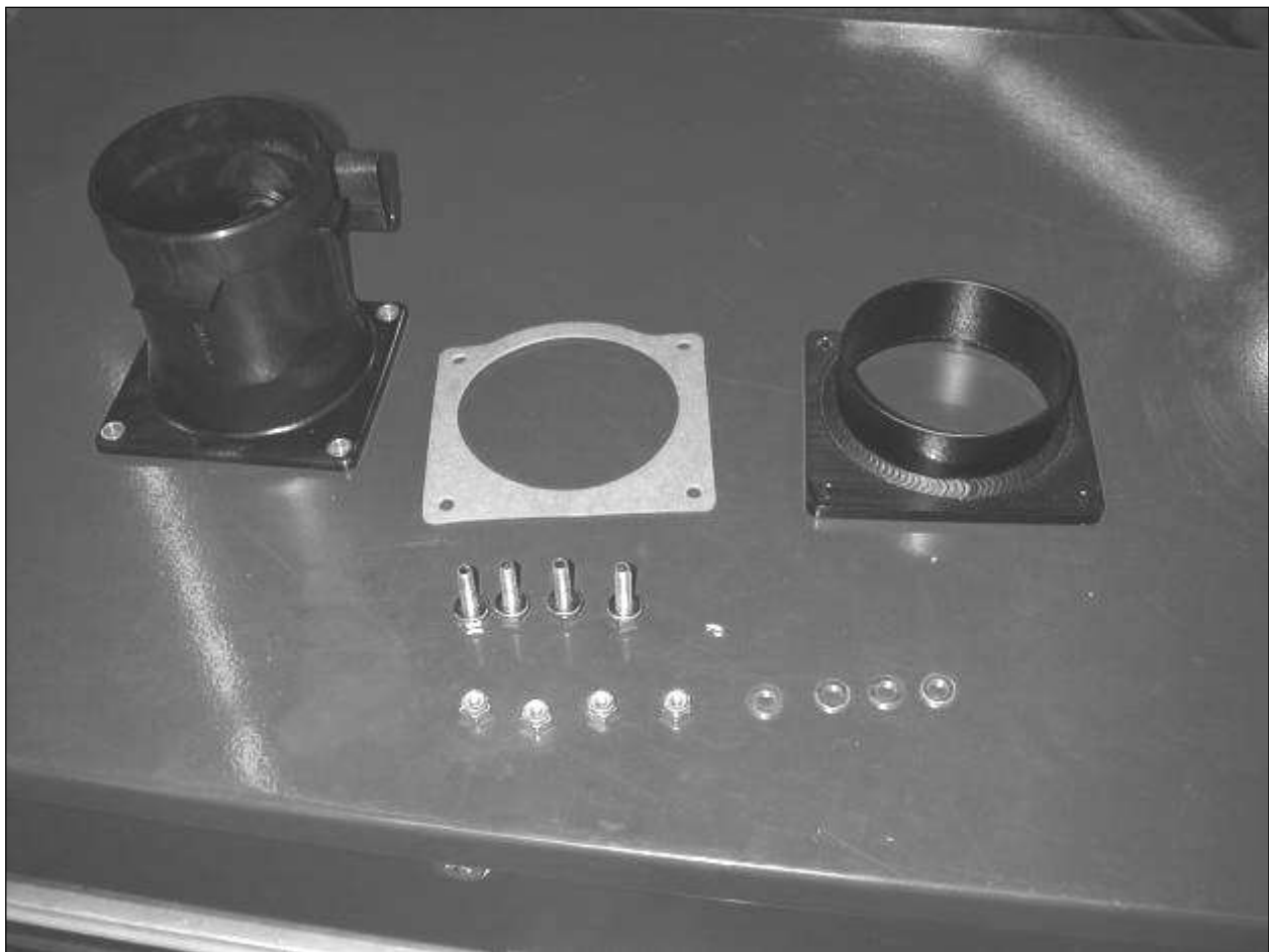
h. The new MAF sensor assembly will contain the above hardware. 1 MAF sensor, 1 gasket, 4 M6x20 bolts, 4 nylok nuts, 4 M6 washers and the MAF sensor adapter.
