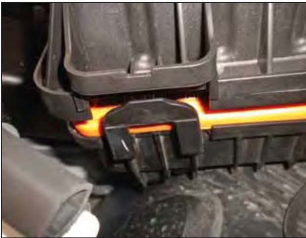
e. Locate the stock air intake system and unclip the 2 plastic tabs retaining the airbox lid.
