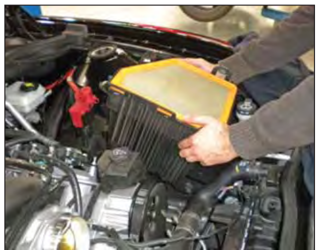
j. Carefully pull up on the lower airbox until it pops free from its retaining anchor. Make sure the rubber anchor stays in the frame rail, it will be needed to properly install the AEM® intake system.
