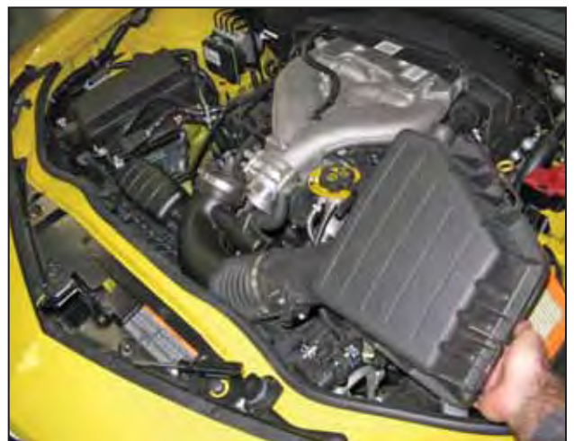
h. Remove the inlet tube and airbox lid from the engine bay. Remember, you will need the factory MAF sensor for your new intake system.
