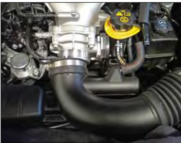
g. Loosen the large hose clamp at the engine throttle body and disconnect the inlet tube.
