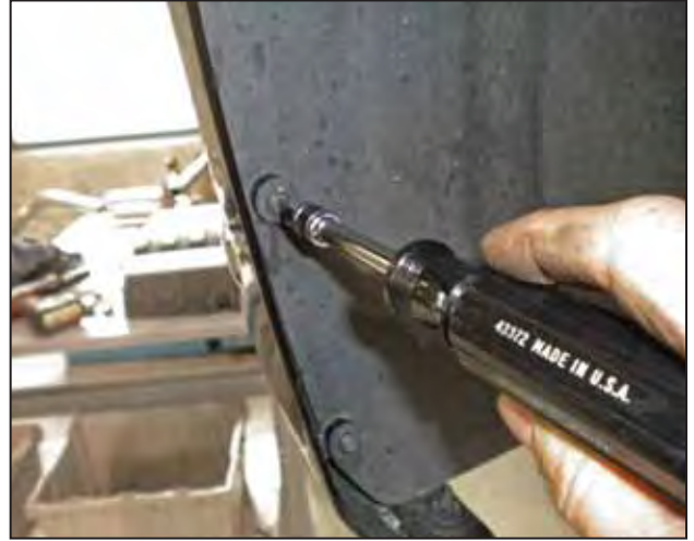
c. Remove the 3 lower Torx T20 retaining screws from the plastic fender well cover.
