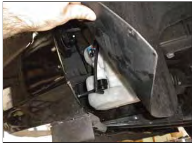
e. Carefully pull the fender well cover away from the fender lip to gain access to the stock washer reservoir.
