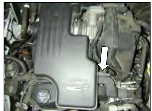
d. Loosen the hose clamp securing the intake resonator to the throttle body. Unplug the small breather hose connected to the front of the intake resonator.
