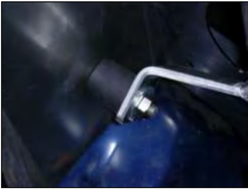
g. Align the intake pipe bracket with the rubber mount on the heat shield. Use the supplied washer and Nylock nut to secure (Do not tighten).
