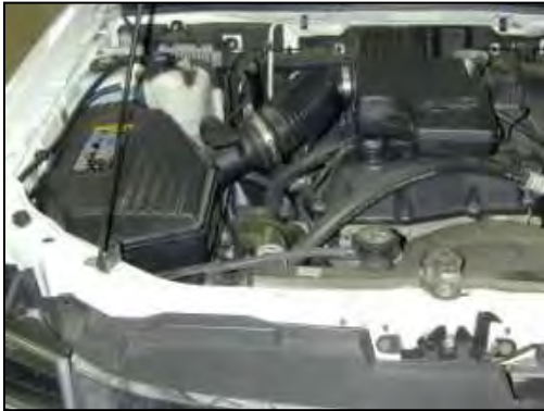
a. Factory airbox system installed.
