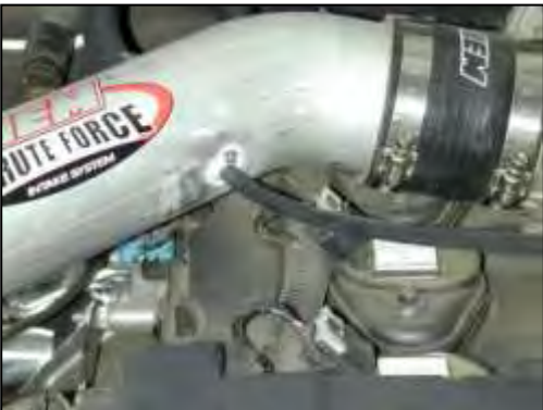
j. Attach the supplied 3/16" vacuum hose between the hard plastic breather hose and the intake pipe.
