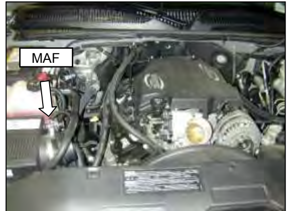
b. Loosen the hose clamp on the rubber elbow attached to the throttle body. Loosen the hose clamp on the MAF sensor and remove the stock plastic intake pipe.
