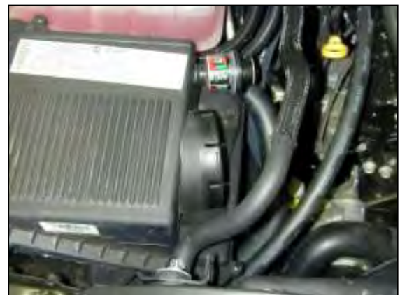
d. Loosen the hose clamp securing the MAF sensor to the stock air filter housing and remove the MAF sensor. Be careful not to damage the sensor!
