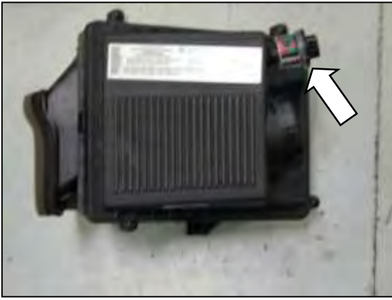
e. Remove the air filter housing by gently lifting up on the inlet pipe of the box. The box is held in with two grommets on the bottom of it. Remove the air filter restriction gauge from the filter housing by gently pulling it out.
