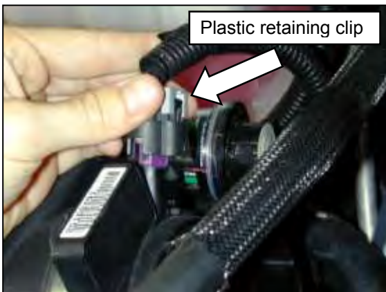
c. Pull back the plastic retaining clip and disconnect the MAF sensor wire harness connector.
