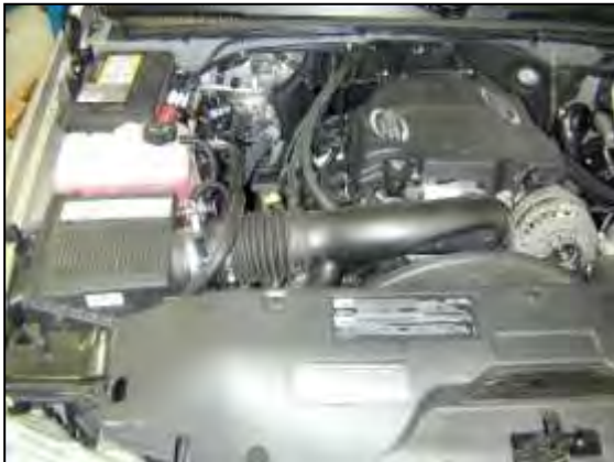
a. Factory airbox system installed.
