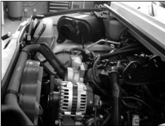
g. Remove the stock air tube from the throttle body up to the air box.
