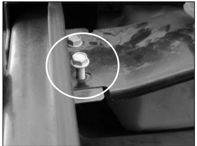
j. Remove bolt closest to the front of the car, near the windshield wiper reservoir.
