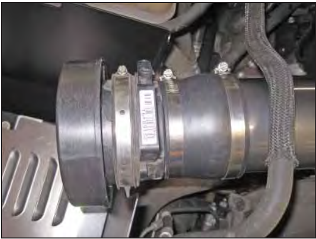
n. Install the MAF sensor assembly created in the previous steps onto the intake pipe.
