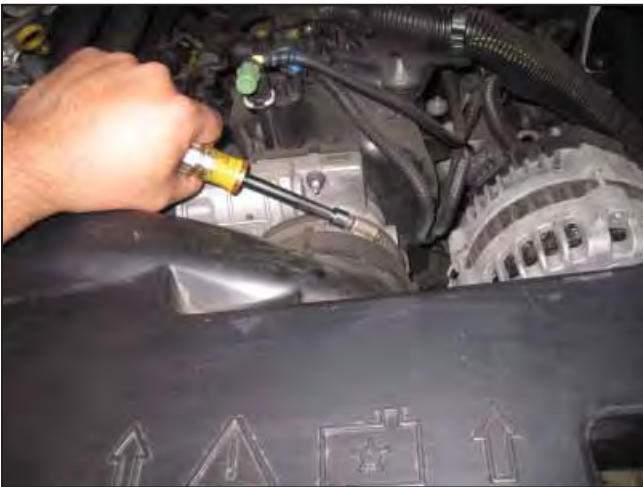
g. Loosen the hose clamp securing the intake duct to the throttle body.
