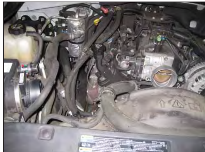
j. Remove the intake duct from the vehicle.
