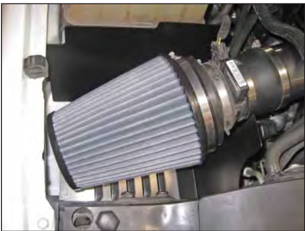
p. Install the air filter on the airhorn.
