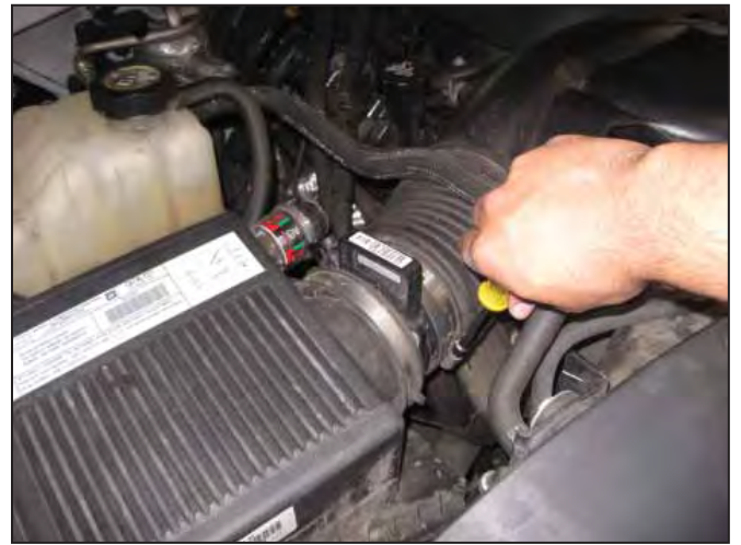
d. Loosen the hose clamp securing the intake duct to the MAF sensor.
