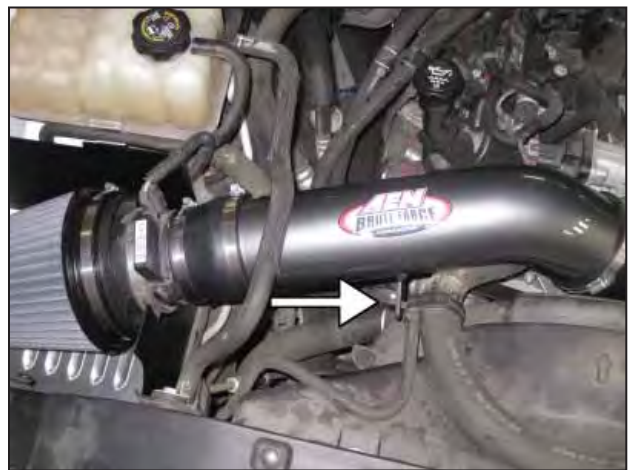
q. Secure the plastic mount on the radiator hose to the intake pipe.
