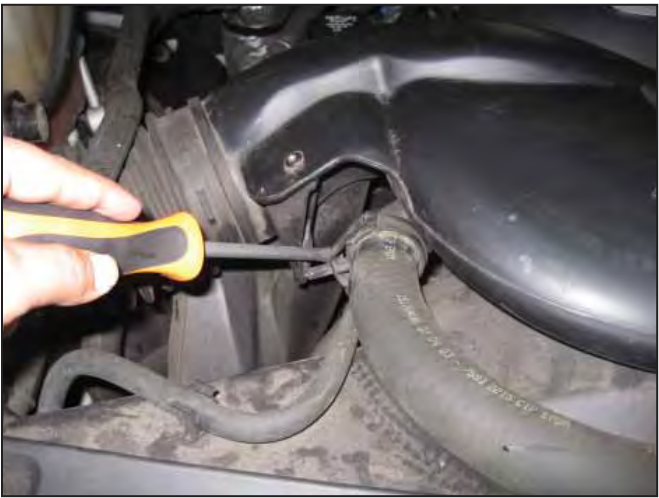
c. Disconnect the plastic mount securing the radiator hose to the intake duct.
