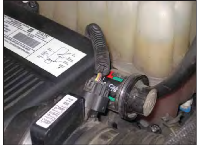
b. Disconnect the mass airflow (MAF) sensor harness.
