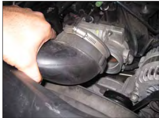
h. Pull the intake duct away from the throttle body.
