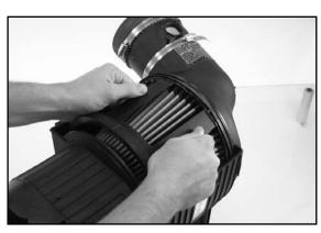
7. Press-fit the filter in the housing as far as possible. Make sure the lug on the bottom of the housing locks the filter in place. It should be in contact with the top ring of the filter.
