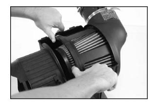
8. To seat the filter in the housing, rotate filter clockwise so the two cavities on the outer ring are facing upward and the filter is in LOCKED position.
