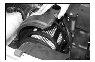
2. Turn the filter counterclockwise so the unlocked cavity is facing upward.
