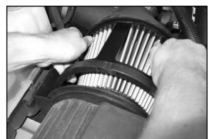
3. Pull filter to front of air box and remove K&N filter.
