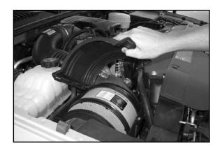
2. Remove the stock air filter from the housing. Care should be taken to dislodge as little dirt as possible.
