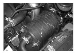
4. Release the four clamps that retains the front and back of air box.
