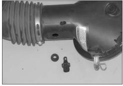
11. On vehicles equipped with an air temperature sensor, remove the air temperature sensor and grommet as shown.
