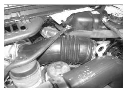
9a. On 2006 and later vehicles, loosen the hose clamp which secures the intake bellows and tube assembly to the turbo inlet.
