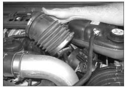
6. Loosen the hose clamp at the mass air sensor, then remove the intake hose from the vehicle.
