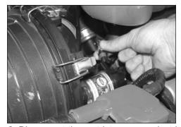
2. Disconnect the restrictor gauge electrical connection as shown.
