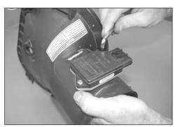
10. On vehicles equipped with a mass air sensor remove the mass air sensor from the factory air box lid with the provided torx wrench as shown.
