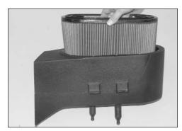
23. Install the K&N air filter into the K&N air box housing as shown.
