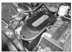
24. Install the K&N air box base and filter into the stock location as shown.
