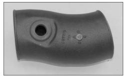
23b. On 2006 and later vehicles, install the provided grommet into the K&N turbo inlet tube as shown.
