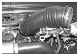
9c. On 2006 and later vehicles, remove the intake bellows and tube assembly from the vehicle as shown.
