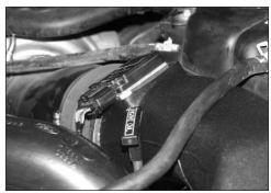
28. On vehicles equipped with a mass air sensor, connect the mass air sensor electrical connection. On vehicles equipped with an air temperature sensor, reconnect the air temperature sensor electrical connection.
