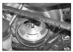
9d. On 2006 and later vehicles, install the silicone hose (08761) onto the turbo inlet and secure with the provided hose clamp.
