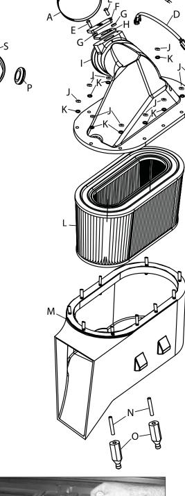
5. Loosen the hose clamp at the turbo inlet tube which secures the intake bellows as shown.
