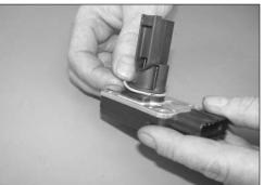
16. On vehicles equipped with a mass air sensor remove the factory O ring from the mass air sensor as shown.
