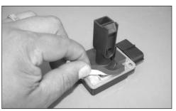
17. On vehicles equipped with a mass air sensor install the provided gasket onto the mass air sensor with the sticky side down.
