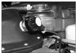
29. Connect the filter minder jumper harness into the filter minder as shown.
