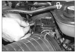
3. On vehicles equipped with a mass air sensor disconnect the mass air electrical connection as shown.
