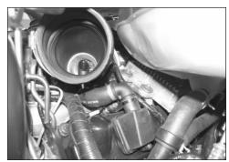
9b. On 2006 and later vehicles, using a large screwdriver, pry up on the crank case vent fitting in the valve cover to disengage it from the valve cover.
