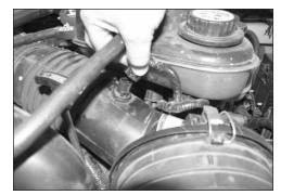
3a. On vehicles equipped with a air temperature sensor, disconnect the temperature sensor electrical connection as shown.
