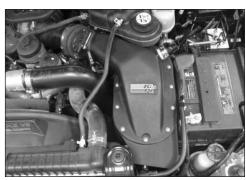
27. Install the K&N air box lid onto the air box base making sure the silicone hose is completely installed onto the throttle body. Install all ten air box lid mounting nuts and washers onto the lid. Once all the nuts are installed they can be tightened completely. Tighten the hose clamp, which secures the silicone hose to the throttle body.
