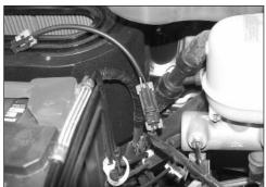
25. Install the provided wiring harness extension to the factory wiring harness filter minder connection as shown.
