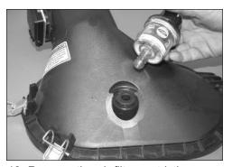
19. Remove the air filter restriction gauge and grommet from the factory air box.
