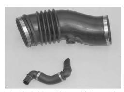
23a. On 2006 and later vehicles, cut the band clamp which secures the crank case vent tube to the turbo inlet tube. Then remove the crank case tube assembly from the turbo inlet tube as shown.
