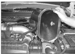
8. Remove the air box base as shown.
