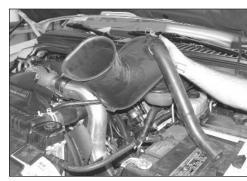
9. Remove the air box top as shown. NOTE: K&N recommends that customers do not discard factory air intake.
