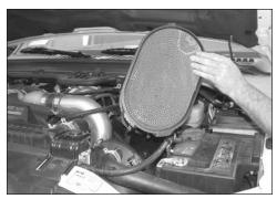
7. Remove the filter housing from vehicle as shown.
