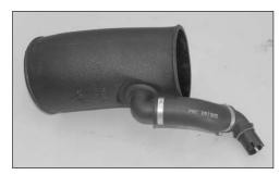
23c. On 2006 and later vehicles, install the crank case vent tube assembly removed in step #23a into the grommet on the K&N turbo inlet tube as shown.
