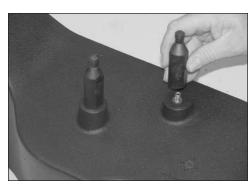
22. Install the two stand off pins onto the two studs installed in step #22.
