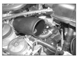
23d. On 2006 and later vehicles, install the K&N turbo inlet tube assembly onto the turbo, rotate to align the crank case vent tube aligns with the vent port in the valve cover. Then snap the crank case vent tube into the valve cover and secure the tube with the provided hose clamp.
