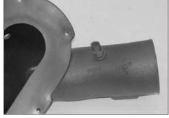
13. On vehicles equipped with the air temperature sensor, install the factory grommet and temperature sensor removed in step #11 into the K&N intake tube at the hole drilled in step #12.
