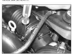
5a. On 2006 and later vehicles, loosen the hose clamp which secures the intake bellows and tube assembly to the rear air filter housing as shown.
