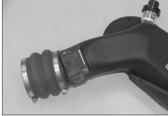
26. Install the silicone hose (08613) onto the K&N air box lid with the provided hose clamp as shown.
