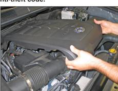
2. Lift up the engine cover to dislodge it from the mounting studs and then remove the engine cover from the vehicle.
