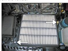
9. Loosen the two bolts securing the lower airbox into the vehicle.
