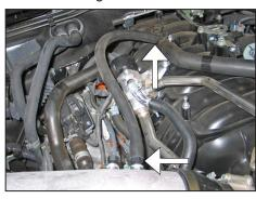
29. Connect the provided crankcase vent line to the NPT fitting and then to the factory TEE fitting on the intake plenum as shown.
