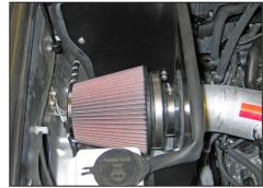
27. Install the filter assembly onto the K&N® intake tube and secure with the provided hose clamp.
