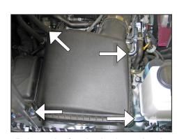
7. Release the four latches' securing the upper airbox to the lower airbox.
