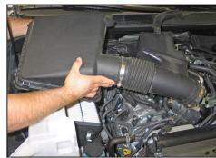
8. Remove the upper airbox/intake hose assembly from the vehicle.
