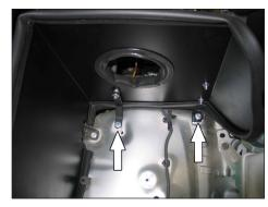
16. Set the heat shield assembly into position on the inner fender. Secure the lower mounting brackets to the inner fender using the factory nut and provided hardware.
