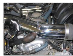
27. Install the engine cover mounting stud into the K&N® intake tube as shown.
