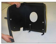
13. Install the provided edge trim around the heat shield as shown.
