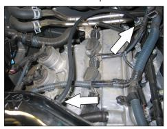
31. Install the provided vacuum hose onto the fuel pressure regulator and then attach the open end to the vent fitting on the  $K\&N^{\otimes}$  intake tube.
