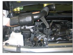
4. Remove the fresh air intake tube from the engine compartment as shown.
