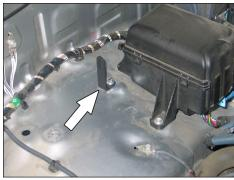
12. Install the "L" bracket (070089) onto the inner fender as shown.
