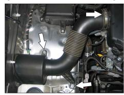
3. Loosen the fresh air intake tube hose clamp and remove the two mounting bolts.
