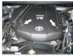
2. Remove the two nuts shown that secure the engine cover and then remove the engine cover.
