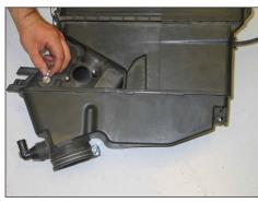
24. Remove the engine cover mounting stud from the factory air box.
