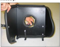
14. Install the provided edge trim inside the opening as shown.
