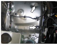
15. Remove the ground strap mounting bolt and the air injection mounting bracket nut shown.
