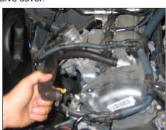
19. Reverse the crank case vent hose and reinstall it back onto the valve cover.
