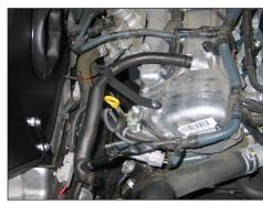
20. Install the tube mounting bracket (070088) onto the valve cover using the provided hardware as shown.
