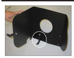
10. Install the "L" bracket (07190) onto the heat shield as shown using the provided hardware. **NOTE: Place the provided spacer**
