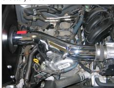
25. Install the K&N® intake tube assembly into the silicone hose at the throttle body and align with the tube mounting bracket, then secure with the provided hose clamp and hardware.
