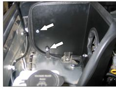
17. Secure the rear of the heat shield to the bracket installed in step #12 using the hardware and spacer provided. Secure the heat shield to the upper bracket with the hardware provided.
