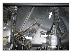
7. Loosen the hose clamp at the throttle body and then remove the two air box mounting bolts shown.
