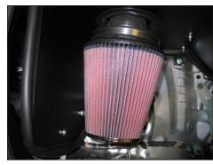
30. Install the filter assembly onto the  $K\&N^{\otimes}$  intake tube and secure with the provided hose clamp.
