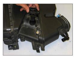
22. Remove the mass air sensor from the stock air box as shown.
