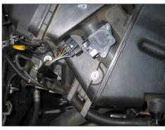
5. Disconnect the mass air sensor electrical connection and unhook the wiring harness from the air box.
