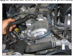
18. Remove the crank case vent hose from the valve cover.
