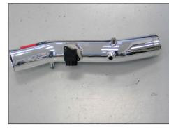
23. Install the mass air sensor into the K&N® intake tube and secure with the provided bolts.
