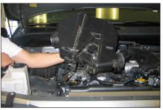
8. Lift up the air box assembly and disconnect the fuel pressure vent line and then remove the complete air box assembly.
