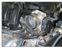
21. Install the provided silicone hose (08711) onto the throttle body and secure with the provided hardware.
