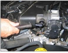
6. Disconnect the crank case vent hose from the air box as shown.
