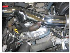
26. Reconnect the crank case vent hose to the K&N® intake tube as shown.
