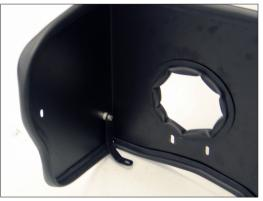
13. Install the provided "C" (#07190) bracket onto the heat shield with the provided hardware as shown.
