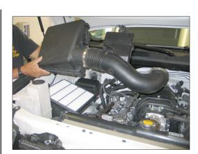
6. Release the four upper air box clam shell clamps, then remove the upper airbox and intake tube assembly.
