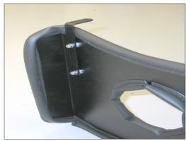
12. Install the long "L" bracket (#070902) onto the heat shield with the provided hardware as shown.
