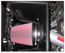
28. Install the K&N® filter assembly onto the K&N® intake tube and secure with the provided hose clamp.
