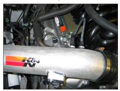
23. Connect the factory fuel pressure vent hose to the K&N® intake tube as shown.
