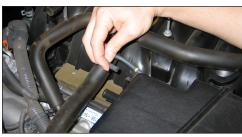
5. Disconnect the fuel pressure regulator vent hose from the stock intake tube as shown.
