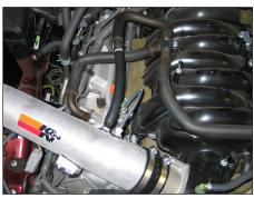
25. Connect the hose mender from the crank case vent hose assembly into the factory crank case vent hose and secure with the factory spring clamp. Then connect the open end to the K&N® intake tube as shown
