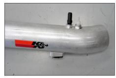
20a. Install the two provided  $\frac{1}{4}$  npt fittings into the K&N® intake tube as shown.
