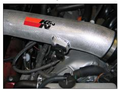
30. Reconnect the mass air sensor electrical connection as shown.
