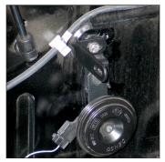
14. Install the small "L" bracket (070742) onto the inner fender using the hardware provided as shown. NOTE: On vehicles equipped with the security system horn, be sure to install the "L" bracket over the horn bracket.
