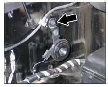
13. On vehicles equipped with a security system horn, remove the bolt which secures the horn to the inner fender.
