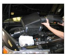
8. Remove the complete stock intake assembly from the vehicle as shown.
