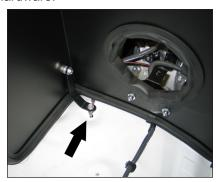
17. Secure the rear lower mounting bracket to the ground strap location with the provided hardware. NOTE: Be sure to place the ground strap between the bracket and inner fender.
