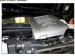
2. Lift up the front of the engine cover and then unhook it from the rear and remove it from the vehicle.
