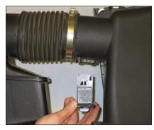
19. Remove the two bolts which secure the mass air sensor into the stock air filter housing and then remove the mass air sensor as shown.
