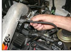
20. Install the provided vacuum hose onto the fuel pressure regulator and then onto the K&N® intake tube as shown.
