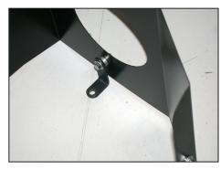
9. Install the small heat shield mounting bracket (070812) with the provided spacer onto the heat shield as shown.
