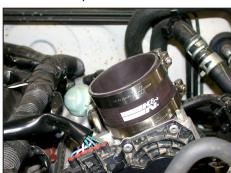
15. Install the provided silicone hose (08440) onto the throttle body and secure with the provided hose clamp.
