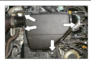
4. Remove the three bolts that secure the intake plenum to the engine and loosen the throttle body hose clamp.
