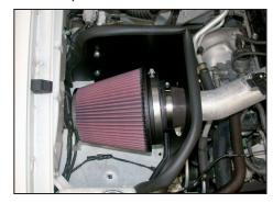
25. Install the air filter assembly onto the intake tube as shown.
