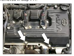
13. Remove the two valve cover bolts shown. **NOTE: These bolts will be reused.**
