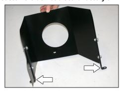
8. Install the two heat shield brackets (07159) onto the heat shield as shown with the provided hardware.
