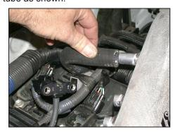
21. Install the provided crank case vent hose onto the valve cover port and then onto the K&N® intake tube as shown.
