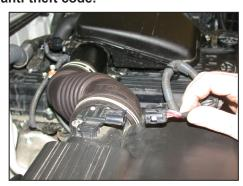
2. Disconnect the mass air sensor electrical connection and unclip the three wire harness retaining clips from the intake plenum.
