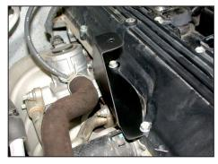
14. Install the tube mounting bracket assembly onto the valve cover using the factory bolts removed in step #13.
