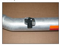
17. Install the mass air sensor into the K&N® intake tube and secure with the provided M4 button head allen bolts as shown.
