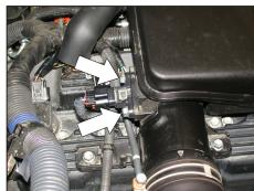
3. Remove the two bolts that secure the pressure sensor to the stock intake tube.
