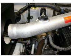
19. Secure the K&N® intake tube to the tube mounting bracket with the provided hardware and then tighten the hose clamp at the throttle body.
