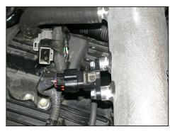
22. Install the pressure sensor onto the K&N® intake tube using the bolts removed in step #3.
