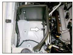
12. Install the heat shield onto the vehicle and secure with the provided hardware and the nut removed in step #11.
