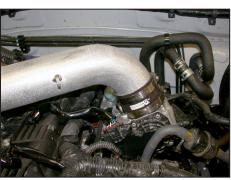
18. Install the K&N® intake tube onto the throttle body and align with the tube mounting bracket that was installed in step #14.
