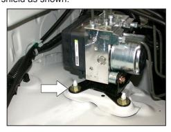
11. Remove the ABS pump mounting nut shown. **NOTE: This nut will be reused.**
