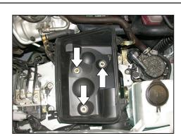
7. Remove the three lower air box retaining bolts shown and then remove the lower air box from the vehicle.
