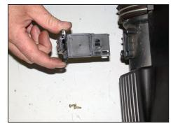
16. Remove the two mass air sensor retaining screws and then remove the mass air sensor from the factory air box.
