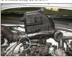
6. Disconnect the wire harness-retaining clip shown from the intake plenum.
