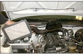
5. Unlatch the upper air box retaining clips, disconnect the fuel pressure regulator and crank case vent hoses and then lift the intake tract off of the throttle body as shown.
