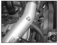
25. Install the original crank case vent hose onto the valve cover, then connect the crank case vent hose onto the K&N® intake tube.
