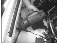
6. Remove the two bolts that secure the resonator to the inner fender, then remove the resonator from the vehicle as shown.
