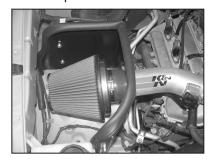
28. Install the  $K\&N^{\otimes}$  air filter onto the intake tube as shown.
