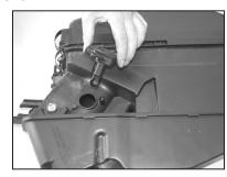
18. Remove the two screws that secure the mass air sensor to the air box assembly, then remove the mass air sensor as shown.
