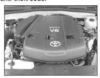
2. Loosen the two nuts that secure the engine cover, then remove the engine cover.
