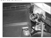
9. Remove the fuel pressure regulator hose from the back side of the air box.
