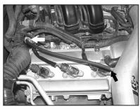
24. Remove the stock vacuum hose from the fuel pressure regulator. Install the provided silicone hose onto the fuel pressure regulator and then attach the opposite end to the K&N® intake tube.
