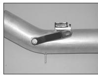
22. Install the provided tube-mounting bracket onto the K&N® intake tube with the provided hardware as shown.
