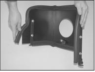
14. Install the provided edge trim onto the heat shield as shown.
