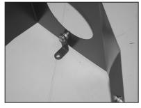
13. Install the small heat shield mounting bracket (070812) with the provided spacer onto the heat shield as shown.
