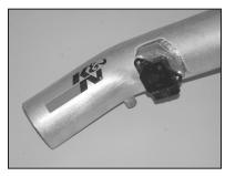
19. Install the mass air sensor into the K&N® intake tube as shown using the provided hardware.
