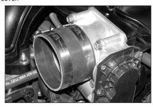
20. Install the provided silicone hose (08434) onto the throttle body with the provided hose clamps.
