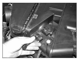
7. Disconnect the two mass air wire harnesses retaining clips from the airbox, then disconnect the mass air sensor electrical connection.
