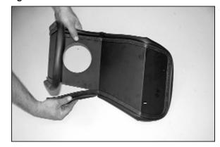
16. Install the edge trim onto the heat shield as shown. Trim if needed.
