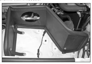
17. Install the heat shield onto the vehicle, then secure the brackets with the provided hardware.
