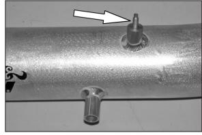
24. Install the stud removed in step #23 into the threaded boss on the K&N® intake tube as shown.
