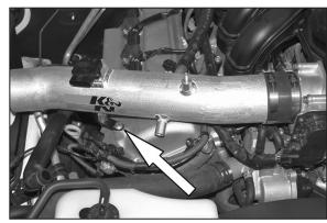
26. Install the K&N® intake tube onto the throttle body, align the mounting bracket with the threaded boss on the engine valve cover and then secure with the provided hardware and hose clamp.
