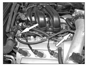
27. Remove the stock vacuum hose from fuel pressure regulator. Install the provided silicone hose, attaching the hose to the fuel pressure regulator and the K&N® intake tube nipple.
