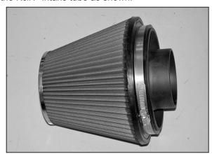
29. Install the filter adapter into the air filter as shown, secure with the provided hose clamp.
