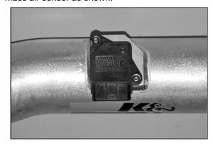
22. Secure the mass air sensor to the K&N<sup>®</sup> intake tube using the provided bolts as shown.
