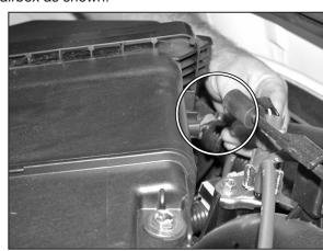
9. Remove the fuel pressure regulator hose from the back side of airbox.
