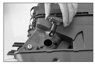
21. Remove the two screws that secure the mass air sensor to the airbox assembly, then remove the mass air sensor as shown.
