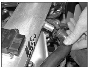
28. Connect the factory crankcase vent hose onto the K&N® intake tube as shown.
