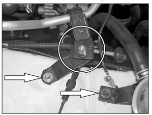
12. On vehicles equipped with the A/C mounting bracket, remove the A/C mounting bracket and loosen the nut. Then, remove the power steering reservoir mounting bolt.
