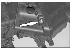
23. Remove the engine cover mounting stud shown from the factory airbox.
