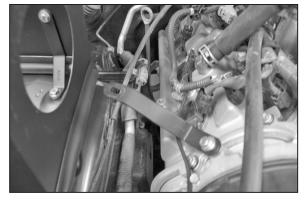
12. Install the tube mounting bracket onto the threaded boss on the cam cover with the provided hardware.
