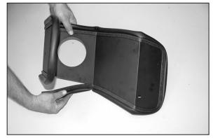
10. Install the edge trim onto the heat shield as shown. Trim if needed.
