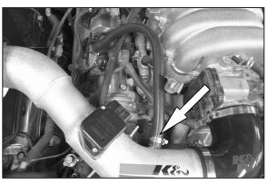
17. Remove the factory crank case vent hose from valve cover and then install the supplied vent hose onto the valve cover and K&N® intake tube and secure with the supplied hose clamp as shown.
