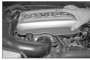
2. Loosen the two nuts that secure the throttle body cover, then remove the throttle body cover
