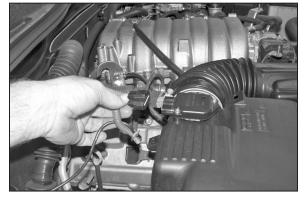
3. Disconnect the mass air sensor electrical connection, then release wire loom from air box.
