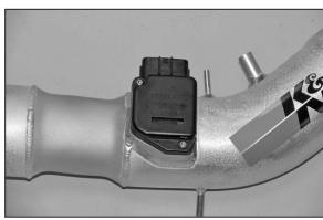
15. Install the mass air sensor into the K&N® intake tube and secure with the provided bolts as shown.
