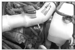
19. Connect the factory power steering pressure switch vent hose onto the K&N® intake tube as shown.
