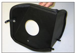
13. Install the heat shield mounting bracket onto the rubber mounted stud installed in step #12 with the provided hardware.
