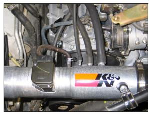
23. Install the one factory P/S vent line, crank case vent line, EVAP vent line, and fuel pressure vent line onto the K&N® intake as shown.
