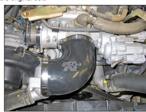
17. Install the provided silicone hose (084095) onto the throttle body with the provided hose clamps.
