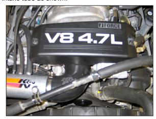
27. Reinstall the throttle body cover and secure with the original nuts.
