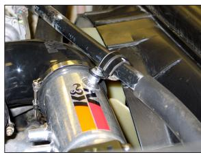
21. Reconnect the A/C line to the K&N® intake tube using the original bolt removed in step #4.
