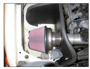
26. Install the air filter assembly onto the K&N® intake tube as shown.
