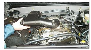
8. Remove the complete air induction system. NOTE: K&N Engineering, Inc., recommends that customers do not discard factory air intake.
