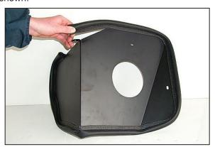
11. Apply the edge trim to the  $K\&N^{\otimes}$  heat shield as shown above, trim if needed.
