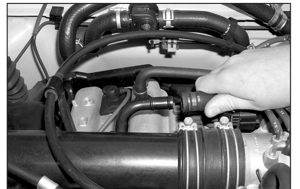
6. Vehicles equipped with an idle air vent line, disconnect vent line as shown.
