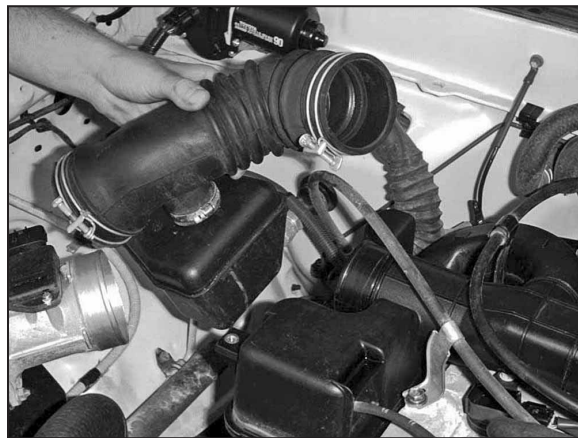
3. Loosen the two hose clamps on the intake hose and remove the intake hose as shown.
