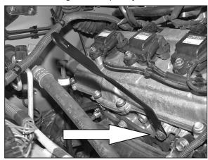
16. Install the tube-mounting bracket onto engine with the supplied hardware as shown.
