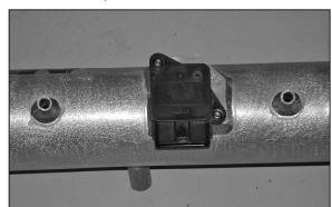
12. Install the mass air sensor into the K&N<sup>®</sup> intake tube and seucre with the provided hardware.
