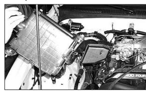
6. Remove the complete air intake system.
