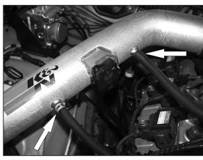
20. Install the provided silicone hose onto the engine and connect it to the K&N® intake tube as shown. Then attach the vent line from EVAP canister to the K&N® intake tube as shown.
