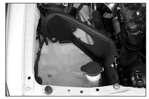
17. Install the heat shield and secure it to the new K&N® brackets with the hardware provided as shown. Do not tighten completely.
