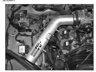
19. Install the K&N® intake tube onto the throttle body and align with the tube mounting bracket installed in step #16. Secure the tube with the provided hardware to the mounting bracket and tighten the hose clamp at the throttle body.
