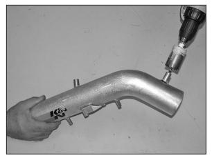
8. On vehicles equipped with the crank case resonator chamber, using a 1-3/8" hole saw, drill out the 5/8" vent port as shown.
