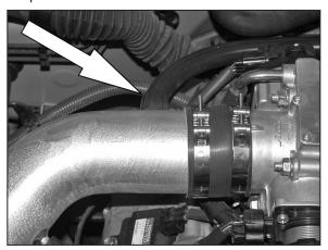
22. On vehicles not equipped with the crank case vent resonator, attach the provided silicone hose onto the crankcase vent and secure with the provided hose clamp. Then connect it to the K&N® intake tube as shown.
