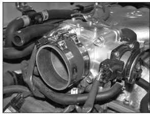
18. Install the silicone hose (08440) onto the throttle body with the provided hose clamps as shown.
