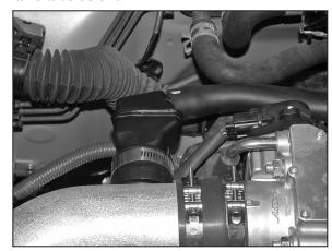
23. On vehicles equipped with crank case vent resonator, connect the factory crank case vent hose onto the resonator as shown.
