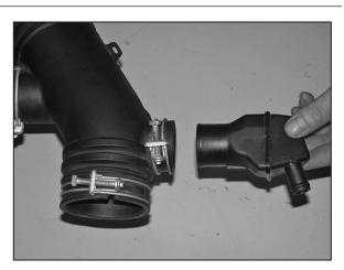
7. On vehicles equipped with the crank case vent resonator chanber, loosen the hose clamp which secures the chanber to the intake tube and remove the chamber from the tube as shown.
