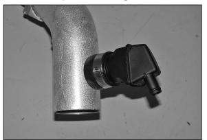
10. Install the crank case venet resonator into the grommet install in step #9 and secure with the provided hose clamp.
