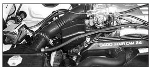
3. Disconnect the three hoses from the air box resonator and intake hose.
