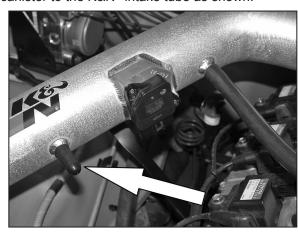
21. On the vehicles that are not equipped with the EVAP canister, use the provided plug on the extra vent port as shown.
