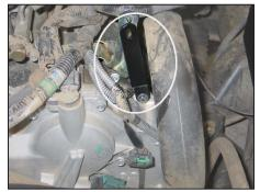
17. Install the tube mounting bracket (07191) onto the engine and secure with the factory bolt removed in the previous step.
