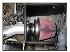
28. Install the filter assembly onto the K&N^ ${\rm \$}$  intake tube and secure with the provided hose clamp.
