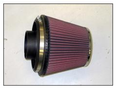
27. Install the filter adapter into the K&N<sup>®</sup> air filter and secure with the provided hose clamp. NOTE: Drycharger<sup>®</sup> air filter wrap; part # RF-1036DK is available to purchase separately. To learn more about Drycharger<sup>®</sup> filter wraps or look up color availability please visit http://www.knfilters.com<sup>®</sup>.
