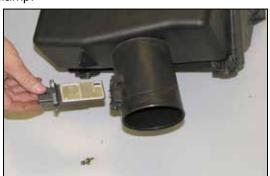
20. Remove the two screws, which secure the mass air sensor to the stock airbox and then remove the mass air sensor from the airbox.
