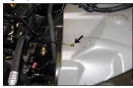
17. Remove the bolt, which secures the ground strap to the inner fender.
