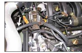
23. Attach the provided silicone crankcase vent hose to the valve cover and  $K\&N^{@}$  intake tube as shown.
