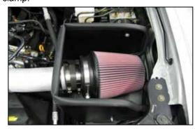
26. Install the air filter assembly onto the intake and secure with the provided hose clamp.
