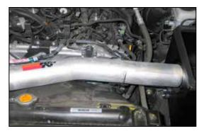
22. Install the K&N® intake tube into the silicone hose at the throttle body and align with the tube mounting bracket installed in step #16. Secure with the provided hardware and hose clamp.
