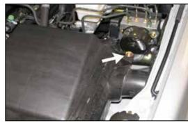
9. Remove the airbox retaining bolt shown.
