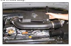
8. Remove the intake tube from the vehicle as shown.
