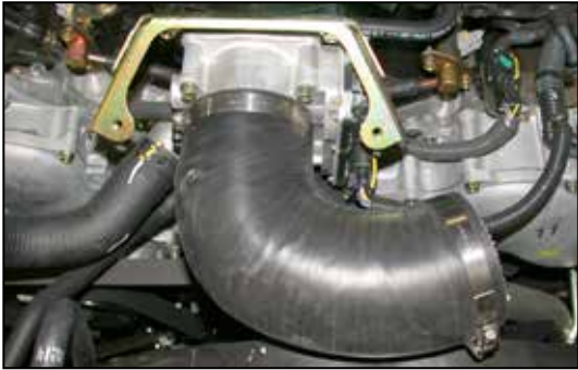
29. Slide the angled hose and hose clamps onto the throttle body, but do not tighten at this time.
