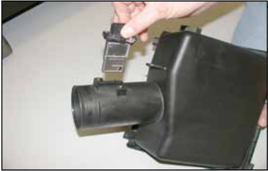
25. Remove the mass air sensor from the air cleaner cover as shown.
