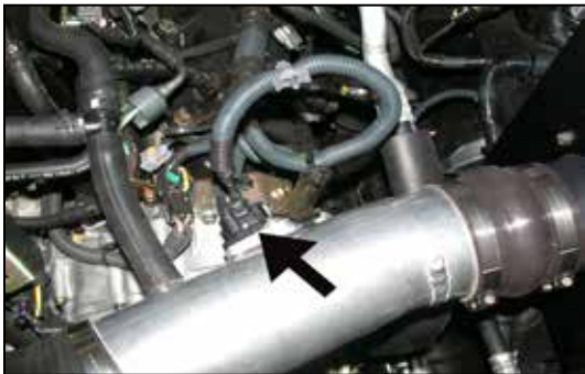
33. Reconnect the mass air sensor electrical connection as shown.
