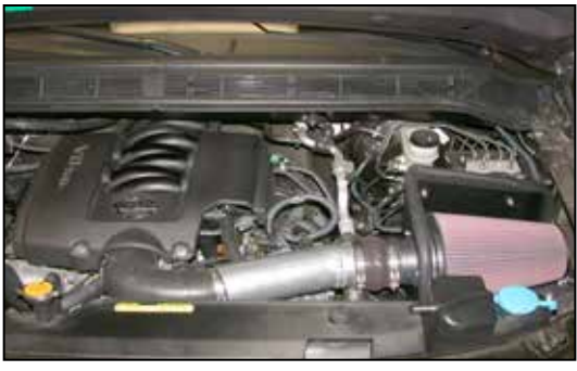
35. Reconnect the vehicle's negative battery cable. Double check to make sure everything is tight and properly positioned before starting the vehicle.
