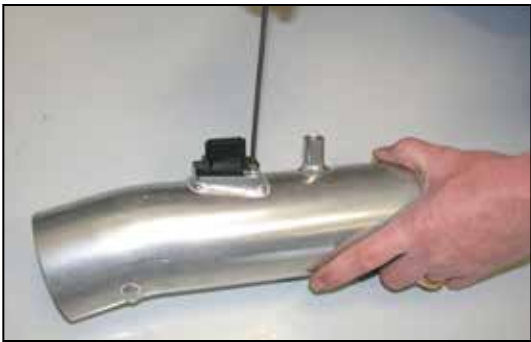
26. Install the mass air sensor into the K&N® intake tube using the provided hardware as shown.
