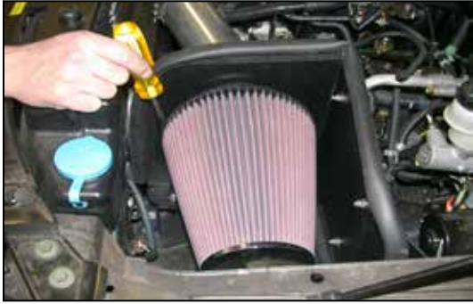
32. Install the K&N® air filter onto the air filter adapter and secure it with the provided hose clamp as shown.
