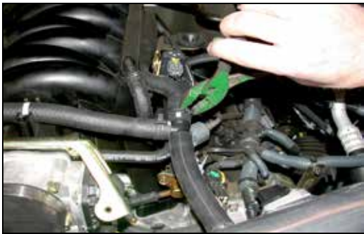
31. Reconnect the crank case vent hoses to the plastic "T" as shown.
