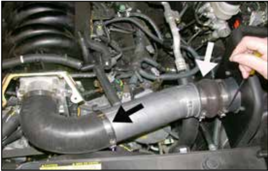
30. Slide the K&N® intake tube onto the filter adapter, then, slide the other end into the angle hose on the throttle body. Adjust everything for best fit, then, tighten all hose clamps as shown.
