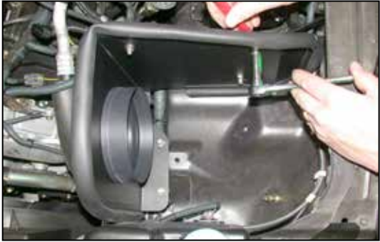
24. Adjust everything for best fit and clearance, then, tighten all hardware at this time.
