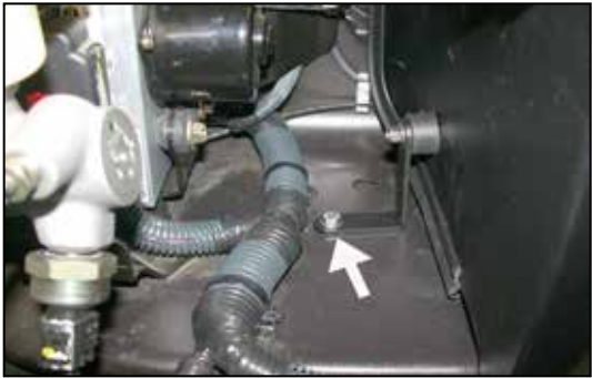
22. Secure the "L" bracket to the hole from step 10 on the inner fender panel with the provided hardware as shown.
