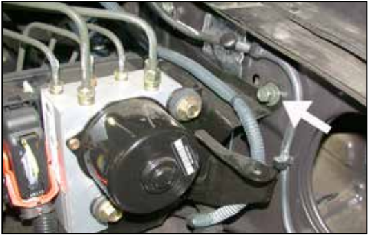
12. Remove the bolt on the ABS bracket as shown.
