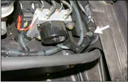
23. Using the bolt from step 12 secure the angle bracket to the ABS bracket as shown.
