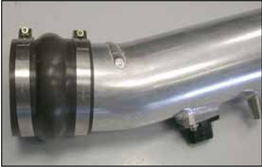
27. Slide the silicone hump hose and hose clamps onto the K&N® intake tube as shown.
