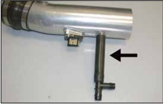
28. Install the provided silicone hose and "T" vent onto the vent on the K&N® intake tube as shown.
