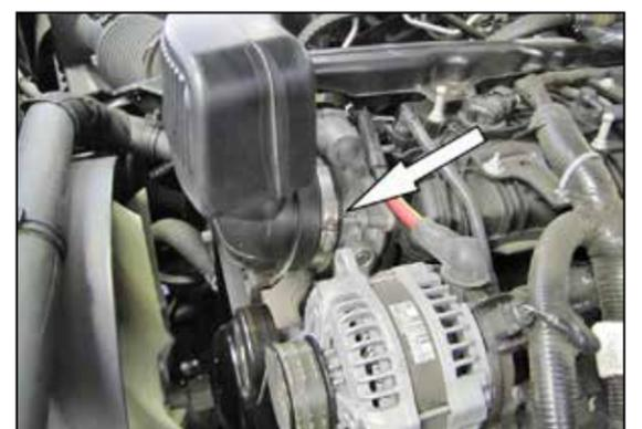
5. Loosen the hose clamps that secure the intake tube to the throttle body and air filter housing. Unhook the radiator hose clip from the intake tube and then remove the intake tube from the vehicle.
