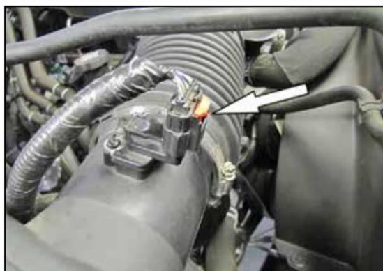
3. Disconnect the mass air sensor and humidity sensor electrical connections.
