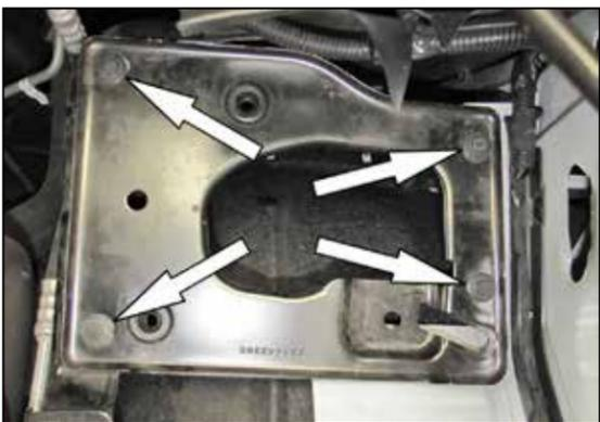
8. Remove the four bolts that secure the air filter mounting tray to the inner fender and then remove the tray.
