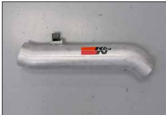
13. Install the mass air sensor and into the K&N® intake tube and secure with the provided hardware.
