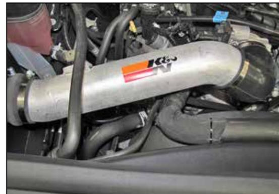
17. Install the K&N® intake tube into the coupling hoses and then adjust the tube for best fit. Secure the hoses and tube with the provided hose clamps.
