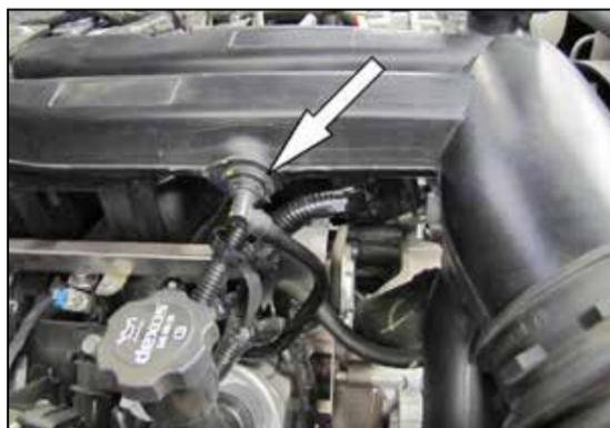
4. Disconnect the crank case vent hose from the intake tube plenum.
