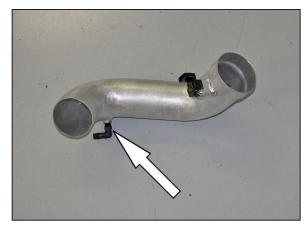
20. Install the provided 90° vent fitting into the  $K\&N^{\circledR}$  intake tube as shown.
