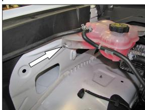
14. Remove the nut that secures the front of the coolant reservoir.
