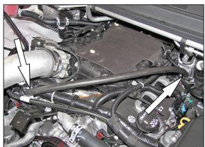
23. Install the crank case vent hose onto the fitting installed into the K&N® intake tube and then connect the hose mender into the fitting on the valve cover.
