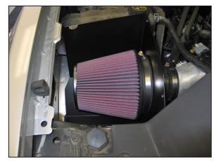
21. Install the K&N<sup>®</sup> air filter and secure with the provided hose clamp.
