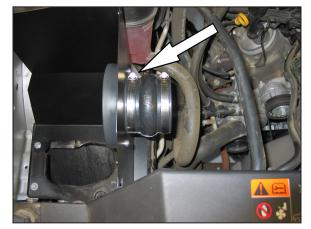
13. Install the provided hump hose (084057) onto the radius adapter and secure with the provided hose clamp.
