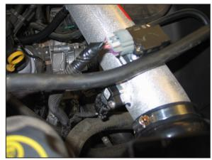
20. Connect the mass air sensor and pressure
