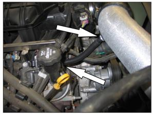
19. Connect the provided crank case vent hose the fitting installed into the K&N<sup>®</sup> intake tube and then connect the open end to the valve cover port.
