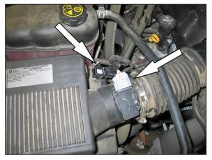
2. Disconnect the mass air sensor and pressure sensor electrical connections shown.
