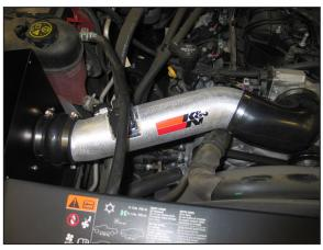
18. Install the K&N<sup>®</sup> intake tube assembly onto the filter adapter and then the throttle body. Adjust the tube and hose for proper fit and then tighten the hose clamps.
