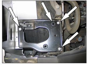
9. Remove the three bolts shown and the rubber grommet shown from the air box mounting plate.
