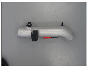
16. Install the sensors into the K&N<sup>®</sup> intake tube and secure with the provided hardware.
