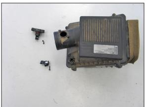
15. Remove the screws securing the mass air
