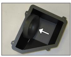
9. Install the provided filter adapter into the K&N® upper airbox and secure with the provided hardware.
