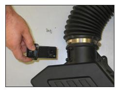
15. Remove the two screws securing the mass air sensor into the factory airbox and then remove the mass air sensor.
