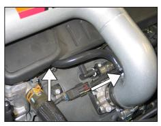
20. Install the provided crankcase vent hose onto the port on the valve cover and then attach the open end onto the vent fitting attached to the intake tube.
