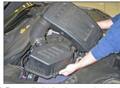
6. Remove the intake plenum and upper airbox from the vehicle.
