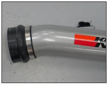
18. Install the provided silicone hose (5-576) onto the K&N® intake tube as shown.
