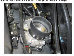
14. Install the provided silicone hose (084034) onto the throttle body and secure with the provided hose clamp.
