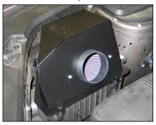
11. Set the K&N® upper airbox assembly onto the factory lower airbox as shown.
