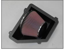
10. Install the K&N® air filter onto the filter adapter and secure with the provided hose clamp.
