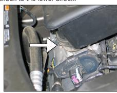
5. Loosen the hose clamp securing the intake plenum to the throttle body.
