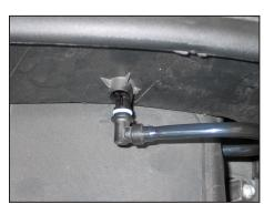
3. Disconnect the crankcase vent tube from the intake plenum as shown.
