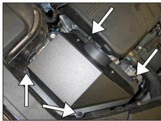
13. Secure the K&N<sup>®</sup> upper airbox with the four screws removed in the previous step.
