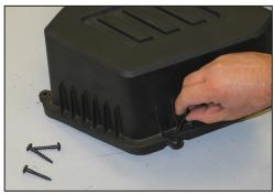
12. Remove the four upper airbox retaining screws from the factory upper airbox.
