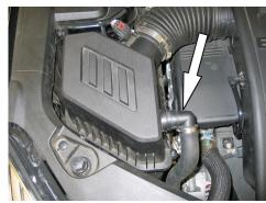
2a. On vehicles equipped with an air injection system, cut the clamp securing the air injection hose to the fitting on the upper air box and disconnect the hose from the fitting.
