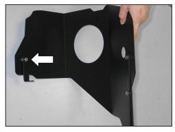
9. Install the small "L" bracket (070602) onto the heat shield using the provided hardware and spacer as shown.
