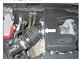
4. Loosen the hose clamp that secures the stock intake tube to the intake resonator.
