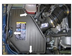
5. Loosen the single retaining nut and two air box retaining bolts.
