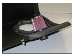
13. Install the provided air pump filter onto the adapter installed in the previous step. Secure with the provided hose clamp.
