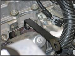
16. Install the tube mounting bracket (06495) onto the cylinder head as shown. Secure with the provided hardware.
