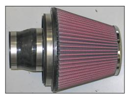
23. Install silicone hose (08724) onto the air filter adapter and secure with the provided hose clamp.
