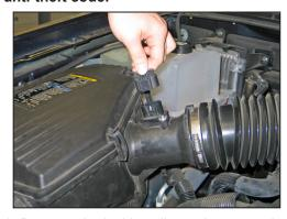
2. Depress the locking clip on the mass air sensor electrical connection, then separate the mass air sensor electrical connection.
