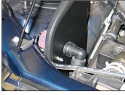
15. Secure the air pump fresh air tube to the adapter as shown.
