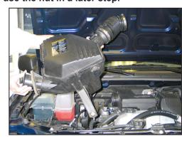
6. Lift the air box up, removing it from the vehicle
