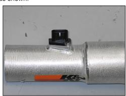
Install the mass air sensor into the K&N $^{\!0}$  intake tube and secure with the provided hardware.
