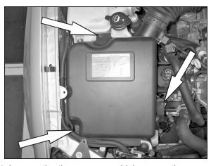
4. Loosen the three screws which secure the upper air box housing.
