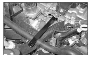
12. Install the tube mounting bracket (26632) onto the engine at the ground cable location and secure with the bolt removed in step #11.
