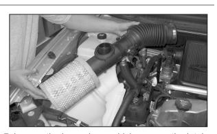
7. Loosen the hose clamp which secures the intake tube to the intake plenum and then remove the complete intake system as shown.
