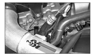
16. Mark the air injection hose at the base of the top 90° bend as shown.
