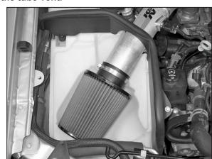
18. Install the K&N® air filter onto the K&N® intake tube and secure with the provided hose clamp. NOTE: Drycharger® air filter wrap; part # RX-4730DK is available to purchase separately. To learn more about Drycharger® filter wraps or look up color availability please visit http://www.knfilters.com®.
