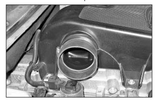
13. Install the provided silicone hose (084091) to the throttle body and secure it with the provided hose clamp.
