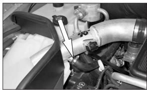
17. Cut the air injection hose at the location marked in step #16. Then install the hose onto the K&N® intake tube and secure with the provided hose
