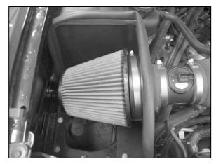
24. Install the K&N® air filter as shown and secure with the provided hose clamp.
