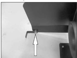
10. Install the "L" bracket (010031) onto the heat shield with the provided hardware as shown.
