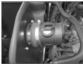
18. Install the mass air sensor assembly into the silicone hose on the filter adapter and secure with provided hose clamp.
