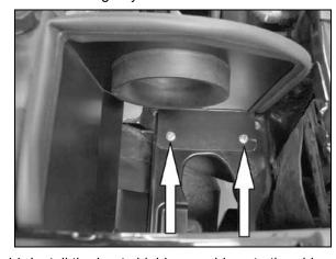
14. Install the heat shield assembly onto the airbox mounting tray and secure to the 5/16" inserted nuts with the provided hardware as shown.
