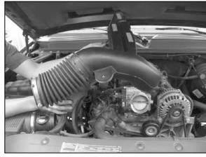
6. Loosen the hose clamps, which secure the stock intake tube to the throttle body and mass air sensor and then remove the intake tube from the vehicle.
