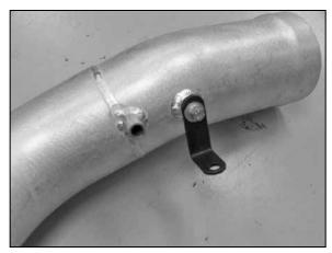
20. Install the "L" bracket (070812) onto the K&N® intake tube with the provided hardware as shown.
