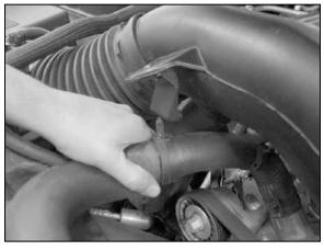
4. Unhook the radiator hose mount from the intake tube.
