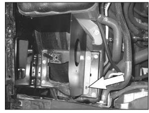
12a. On vehicles that are not equipped with the front airbox mounting grommet and hole, install the heat shield assembly as shown. Then, use a marker to mark the mounting plate through the heat shield mounting hole.
