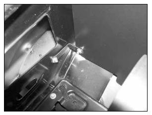
15. Secure the heat shield mounting bracket to the inner fender with the fender washers and hardware as shown.
