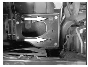
12. Remove the two air box mounting grommets shown.
