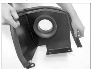
11. Install the provided edge trim onto the heat shield as shown.
