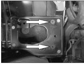
13. Install the two 5/16" inserted nuts into the airbox mounting tray as shown.
