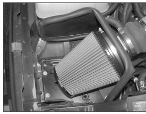
15. Install the K&N® air filter onto the heat shield assembly as shown.
