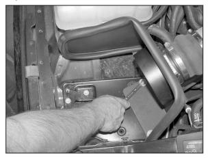
14. Adjust the heat shield and intake tube for best fit, then tighten the two nuts as shown.
