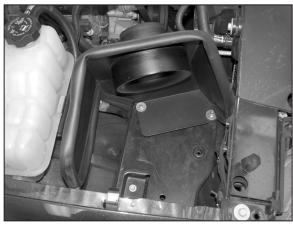
10. Install the heat shield assembly onto the rubber mounted studs using the hardware provided.
