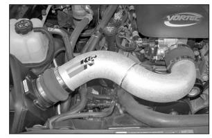
13. Install the K&N® intake tube onto the mass air sensor, then secure the other end onto the throttle body as shown.
