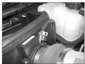
16. Reconnect the mass air sensor electrical connection as shown.
