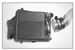
7. Loosen the hose clamp and remove the mass air sensor from the air cleaner.
