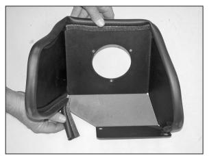
8. Apply the trim seal to the heat shield assembly as shown.
