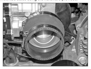
11. Install the silicone hose (08050) and hose clamps onto the throttle body as shown.
