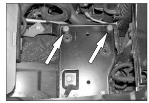
6. Install the rubber mounted studs onto the previous bolt locations removed in step #5
