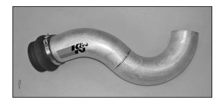
12. Install the silicone hump hose (08176 )and hose clamps onto the K&N® intake tube as shown.
