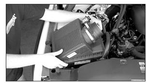
4. Pull firmly upwards to release the air cleaner assembly from the mounting tray grommets, then remove the assembly.
