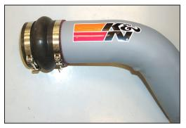
15. Install the silicone step hump hose and hose clamps onto  $K\&N^{\mbox{\scriptsize \$}}$  intake tube as shown.
