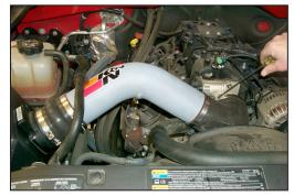
16. Install the K&N<sup>®</sup> intake tube into the angled hose, then, slide the other end into the hump hose. Adjust everything for best fit and clearance and tighten all hose clamps as shown.
