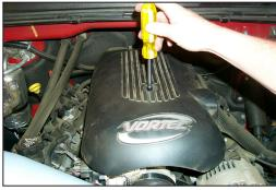
20. Reinstall the engine cover and secure it with the stock hex bolt.
