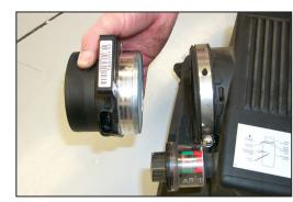
7. Loosen the hose clamp on the air cleaner then remove the mass air sensor as shown.
