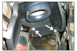
13. Secure the heat shield to the rubber mounted studs using the provided hardware but do not tighten at this time.
