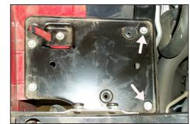
2. Remove the bolt that secures the engine cover, then, remove the engine cover as shown.
