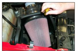
18. Install the K&N<sup>®</sup> air filter onto the mass air adapter and secure it with the provided hose clamp as shown.
