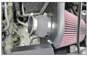
12. Install the provided step hose (084055) onto the filter adapter and secure with the provided hose clamp.
