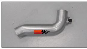
15. Install the inlet air temperature sensor into the K&N<sup>®</sup> intake tube and secure with the hardware provided.
