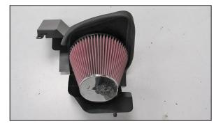
10. Install the K&N<sup>®</sup> air filter onto the filter adapter and secure with the provided hose clamp. NOTE: Drycharger<sup>®</sup> air filter wrap; part # RF-1048DK is available to purchase separately. To learn more about Drycharger<sup>®</sup> filter wraps or look up color availability please visit http://www.knfilters.com<sup>®</sup>.
