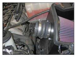
15. Install the provided silicone hump hose (5-576) onto the filter adapter and secure with the provided hose clamp.
