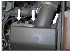
3. Release the three upper air box retaining clips.
