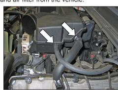
6. Disconnect the crank case vent line and EVAP vent line from the intake plenum.
