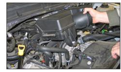
8. Unhook the heater hose clip from the intake plenum and then remove the plenum from the vehicle.
