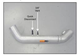
16. Install the quick disconnect and 3/8 NPT vent fittings into K&N® intake tube as shown.
