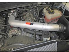
19. Install the K&N® intake tube into the silicone hose at the air filter and then into the silicone hose at the throttle body and secure with the provided hose clamps.
