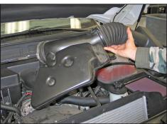
5. Remove the stock intake tube, upper air box and air filter from the vehicle.
