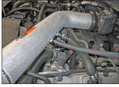
20. Connect the crank case vent hose and EVAP vent hose to the K&N® intake tube.
