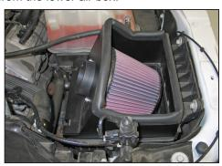
13. Install the K&N® filter/heat shield assembly and secure with the two remaining factory upper air box retaining clips.
