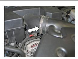
4. Loosen the hose clamp securing the intake tube to the intake plenum.
