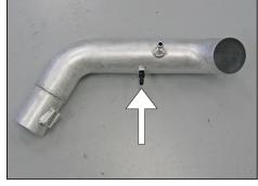
16. Install the provided 3/8" hose fitting into the  $K\&N^{@}$  intake tube as shown.
