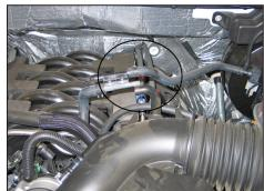
4. Disconnect the EVAP hose from the check valve as shown.
