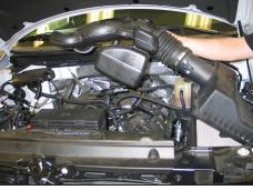
6. Release the three clips securing the upper air box housing to the lower housing and then remove the intake tube/upper airbox and air filter from the vehicle.
