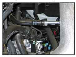
20. Connect the crankcase vent hose to the quick disconnect fitting on the K&N® intake tube.
