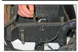
12. Remove the center airbox retaining clip.
