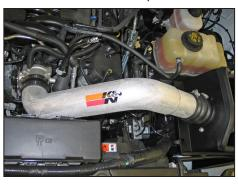
19. Install the K&N® intake tube assembly into the silicone hose attached to the filter adapter and then into the silicone hose on the throttle body. Secure with the provided hose clamps.
