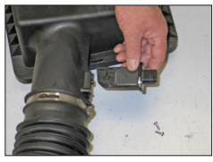
17. Remove the two screws securing the mass air sensor, then remove from the stock intake tube as shown.
