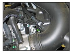
3. Rotate the locking tab and then unhook the crankcase vent hose from the factory intake tube.
