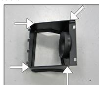
10. Install the two 9" sections of edge trim onto the bottom of the heat shield as shown.
