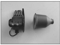
9. Unlatch the clam shell connector and separate the air filter assembly as shown.
