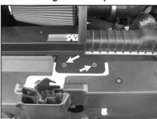
31. Using the factory bolts removed in step #5 secure the heat shield to the radiator core support.
