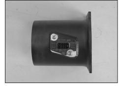
14. On 2006 models, install the mass air sensor removed in step #13 into the mass air sensor housing with the supplied hardware as shown.
