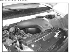
2. Unhook the fresh air intake scoop from the radiator core support and then rotate it back to unlock from the air filter assembly. Then remove it from the vehicle.
