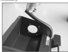
16. Install the long edge trim to the heat shield as shown. Some trimming of the edge trim may be necessary.
