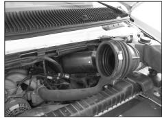
8. Remove the intake tube from the vehicle.
