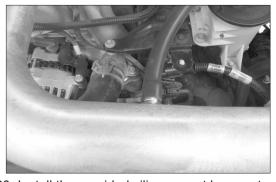
20. Install the provided silicone vent hose onto the valve cover and onto the K&N<sup>®</sup> intake tube as shown.
