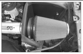
23. Install the filter assembly onto the  $K\&N^{\otimes}$  intake tube and secure with the provided hose clamp.
