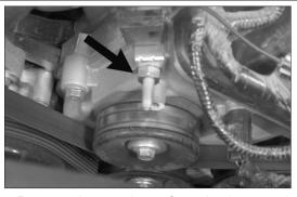
17. Remove the nut shown from the 8mm stud protruding from the engine. **NOTE: This nut will be reused.**
