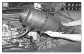
5. Pull firmly up on the air filter assembly to remove it from the mounting grommets.
