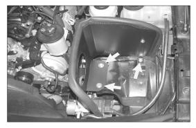
10. Install the heatshield as shown and secure with the provided hardware.
