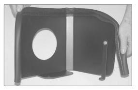
7. Install the edge trim onto the heatshield as shown. Trim if needed.
