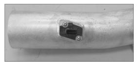
15. Install the mass air sensor assembly into the  $K\&N^{\ensuremath{\mathbb{R}}}$  intake tube and secure with the factory mounting bolts.
