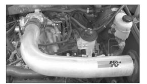
19. Install the K&N<sup>®</sup> intake tube into the silicone hose at the throttle body and align with the mounting bracket and secure with the provided hose clamp and hardware.
