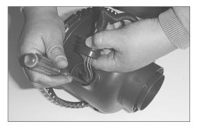
12. Slide the rubber grommet back and disconnect the primary mass air sensor electrical connection, using a flat blade screwdriver.
