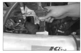
24. Reconnect the secondary mass air sensor electrical connection and then reconnect the mass air sensor primary electrical connection.
