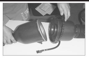
11. Open the air cleaner assembly and isolate the mass air sensor assembly.
